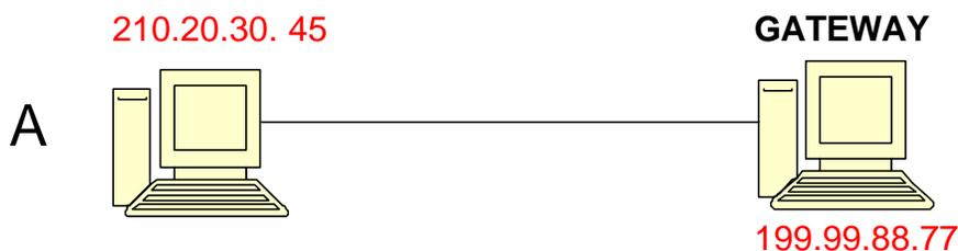
The netmask for A may be set to 255.255.255.255, indicating no other nodes on the local network, and the gateway is set to 199.99.88.77. A default route must be set up at Node A as well, which provides the route for all packets whose destination does not correspond to any specific routing entries.
